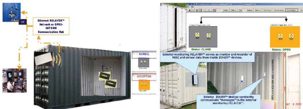
Fig. 5. AVANTE container security device information flow
